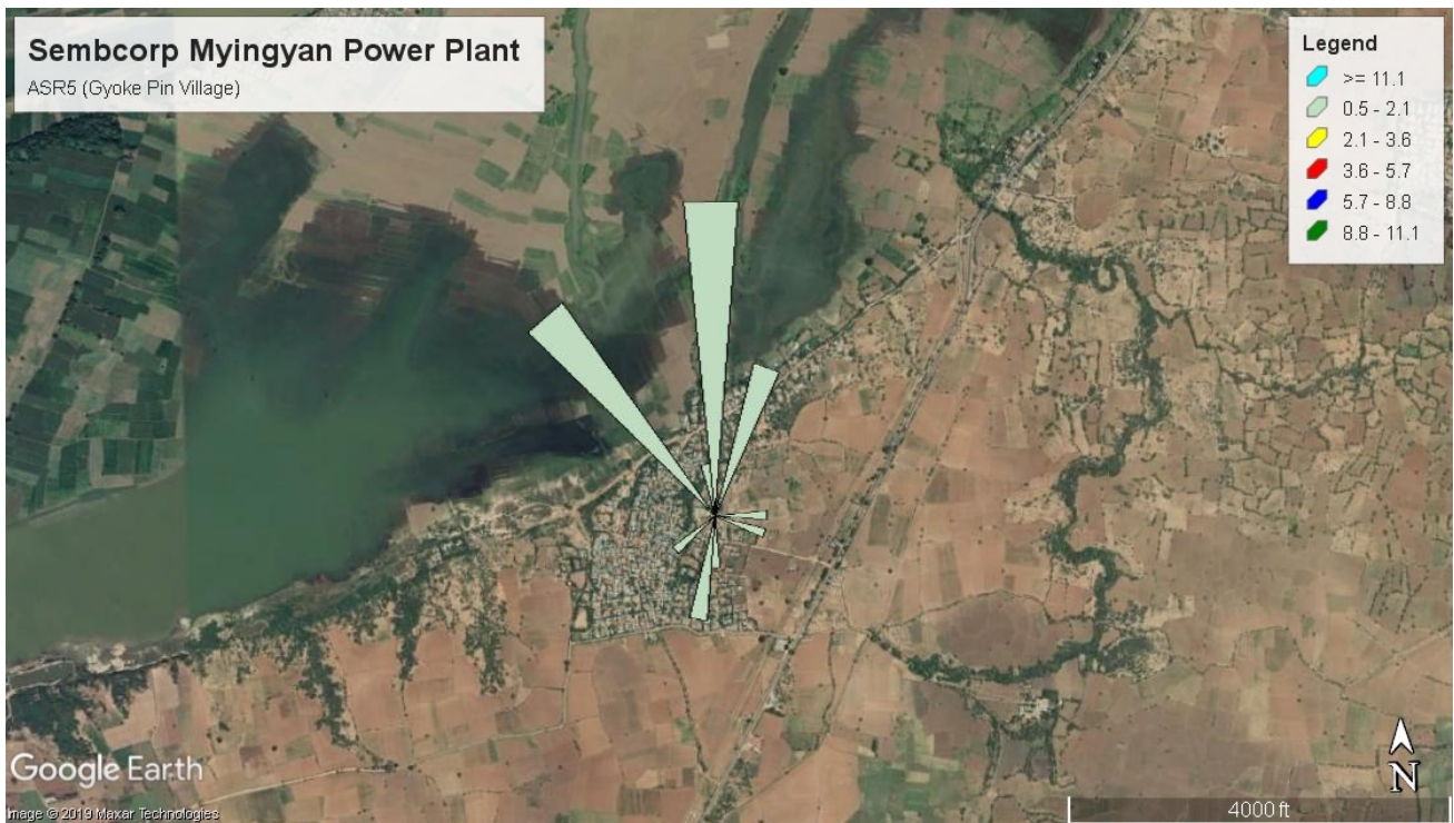
Figure 4. 13 Wind Speed and Wind Direction (Blowing From) at Gyoke Pin Village (ASR5)
