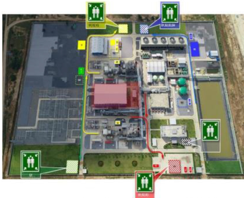
Emergency escape routes and assembly areas were highlighted since conducting SIC for all.
