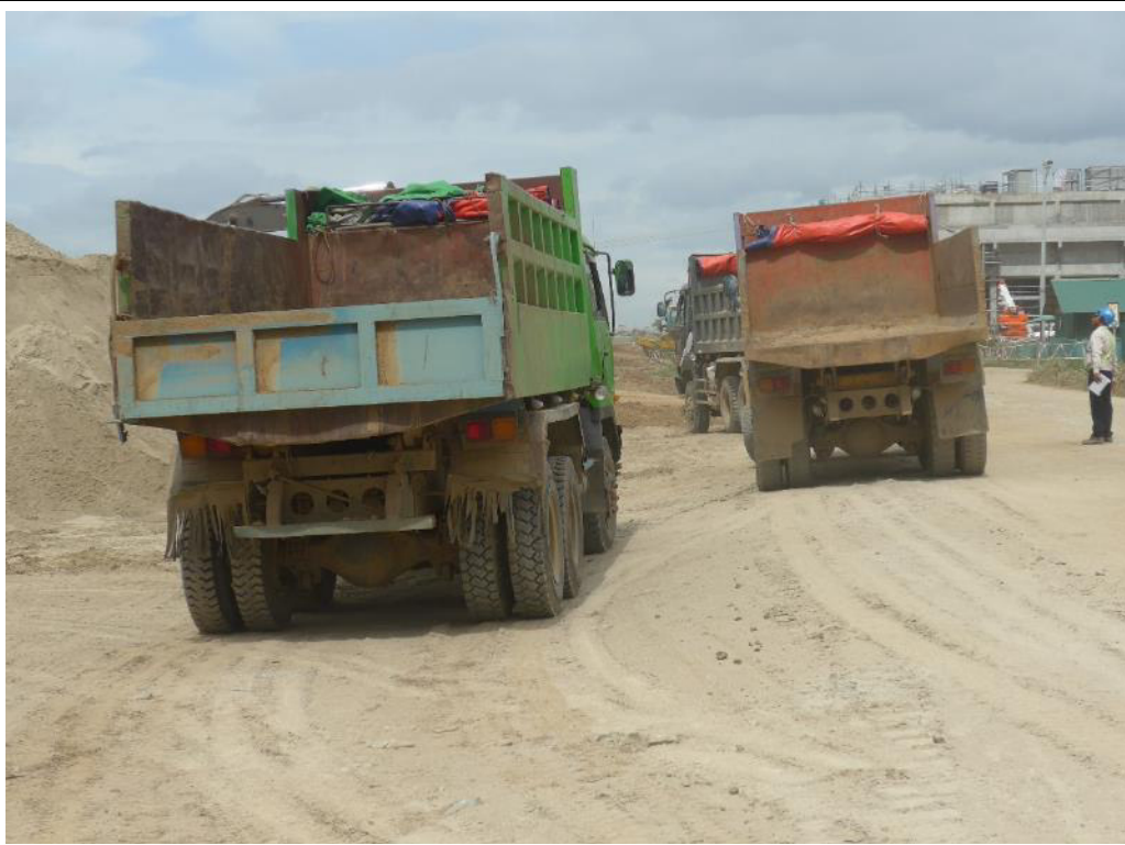
Photo 4: Trucks fitted with covers that are used when conveying soil and dusty materials
