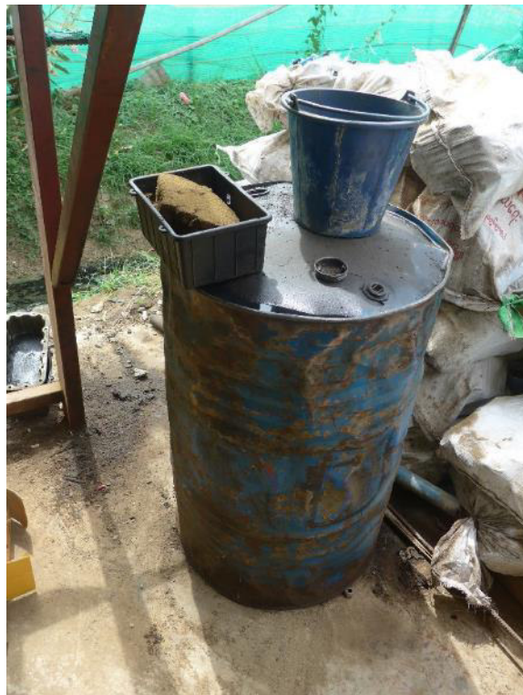
Photo 24: Oil drum in poor condition, with adjacent ground staining
