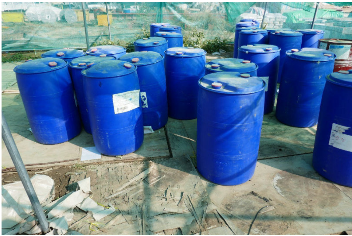
Photo 25: Some chemical storage drums are deformed from exposure to sunlight
