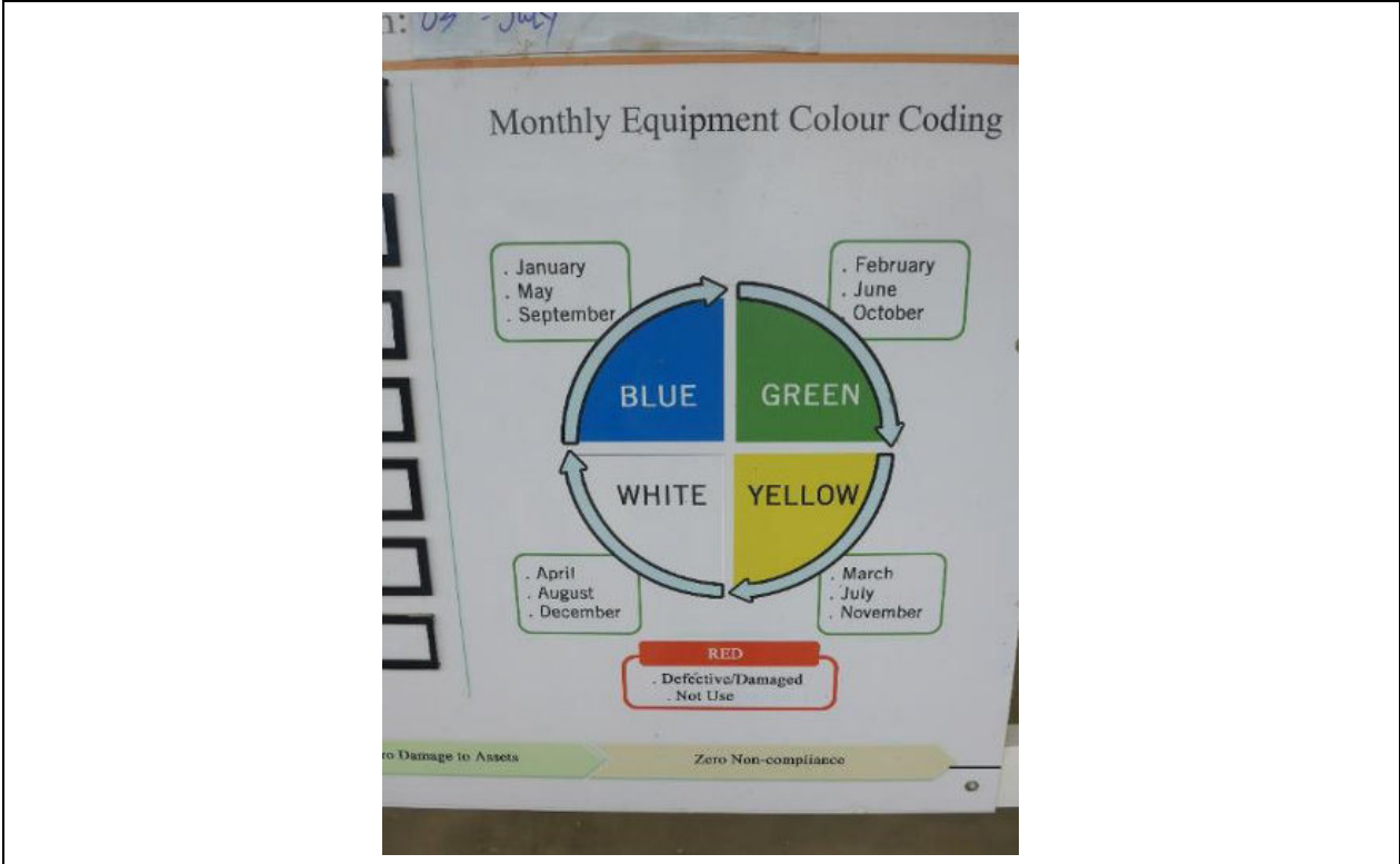
Photo 6: Equipment colour-coding to demonstrate maintenance and fitness-for-use
