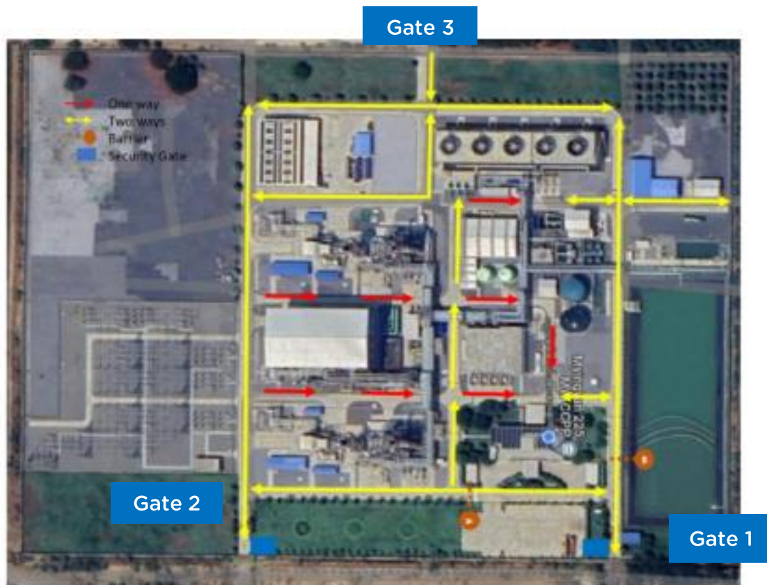
Figure 5-3: Site Traffic Flow for Operations Phase
